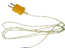
SONDE THERMOCOUPLE K
